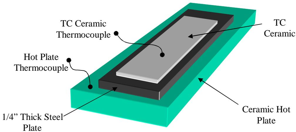
using a dry film thickness gage and then marked on the surface of the TC Ceramic. The samples were then placed on a ceramic hot plate and the surface temperatures of the ceramic hot plate and the TC Ceramic were measured using a Type K Beaded-wire Thermocouple. The thermocouples were placed on the surface of both substrates, with the beaded-wire in intimate contact with the substrate (see Graphic 1).
